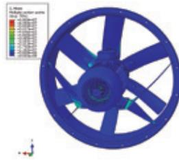
The cast aluminium's fatigue limit for 28.8 million cycles is about 80 MPa. All Aluminium parts have a stress below 65 MPa, so all this parts meet the requirements. The steel's fatigue limit is much higher than aluminium, so all steel parts meets too the requirements.
