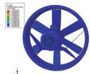
The test result confirms that the fan can resist the impact required by the standard, because 23.5 MPa is a stress value too low for steels.
