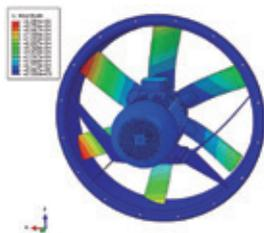
Fan's stress map after the test. The maximum stress is 69.7 MPa for steel parts and 65 MPa for aluminium parts. It is the maximum for all axes.
