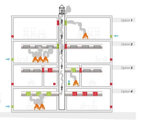
Pressurisation system for stairs, halls and evacuation routes, complemented by smoke exhaust system
